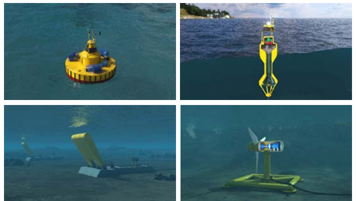
In 2022, NREL released six animations, including (clockwise from top left): Research Reef (observation buoy), Tidal Town (tidal turbine), Desalination Station's surge flap, and the island's Navigation Network (navigation buoy).
