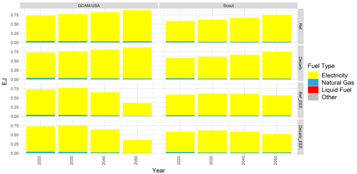
Figure 50. Commercial building energy consumption for cooling by fuel, year, model, and scenario, 2020–2050 (GCAM-USA and Scout)
