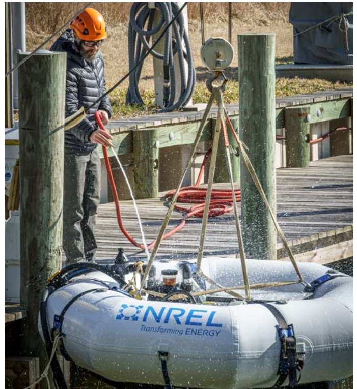
Scott Jenne prepares NREL's hydraulic and electric reverse osmosis wave energy converter device for its ocean outing in North Carolina. Photo by Andrew Simms, NREL
