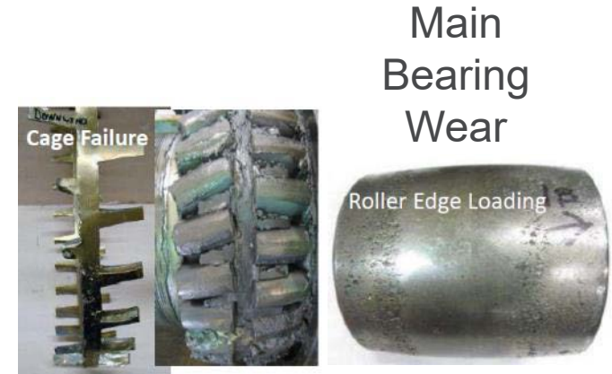
D. Brake. WTG SRB Main Bearing Failures. Presented at the 2013 UVIG Wind Turbine/Plant Operations & Maintenance Users Group Meeting.
