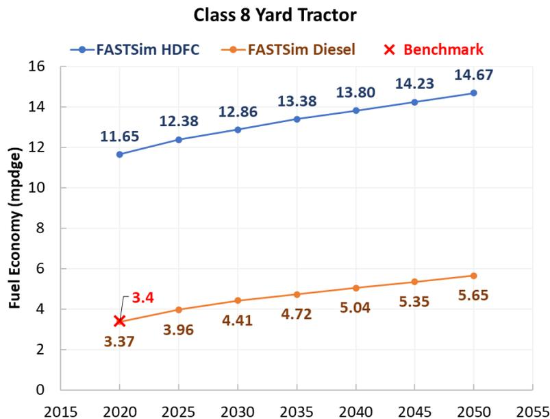
**Figure 19. Fuel economy projections out to 2050 for Class 8 Yard Tractors (200-mile range) for conventional diesel and HDFC powertrains.**
