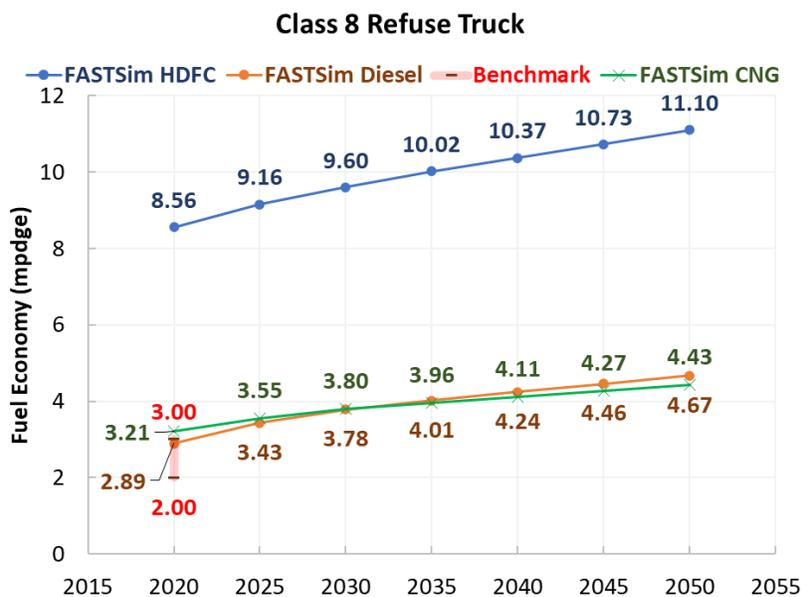
Figure 20. Fuel economy projections out to 2050 for Class 8 Refuse Trucks (200-mile range) for conventional diesel, CNG, and HDFC powertrains.
