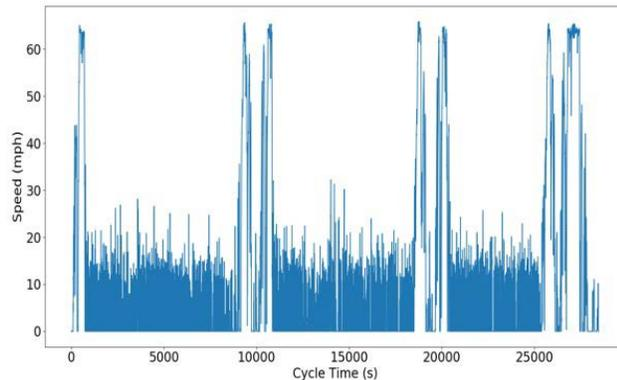
**Figure 13. Representative duty cycle for the Class 8 refuse truck with accompanying duty cycle attributes and metrics. \*Note the sections of the duty cycle below a speed of 30 mph pertain to the truck's trash collection period while the sections approaching 60 mph reference the time that the refuse truck is traveling from one collection zone to the next.**
