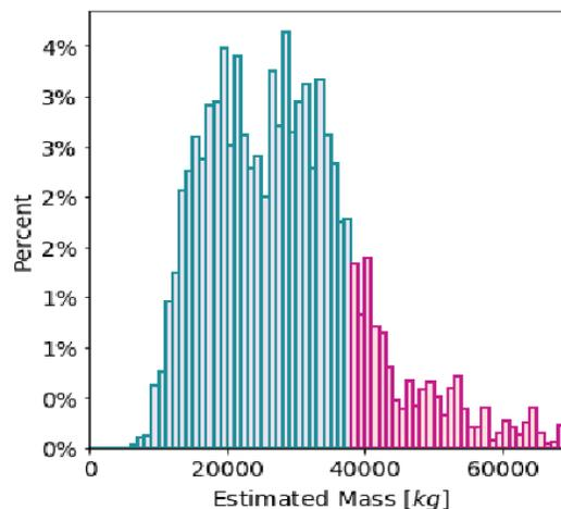
**Figure 10. Estimated total yard tractor mass (tractor + cargo) based on NREL Fleet DNA data and duty cycle used in this analysis (Kotz et al. 2020).**
