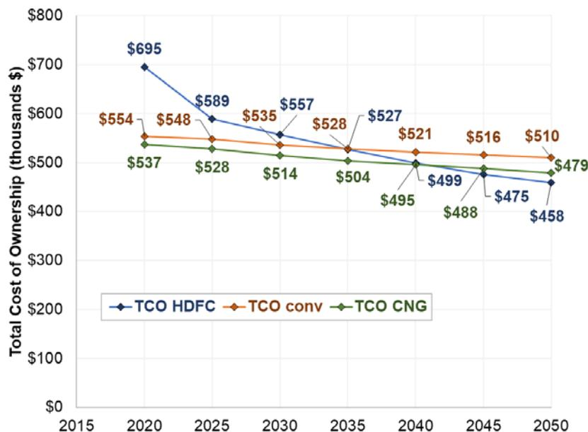
Figure 26. Total cost of ownership comparison for the conventional diesel, CNG, and HDFC Class 8 refuse trucks.
