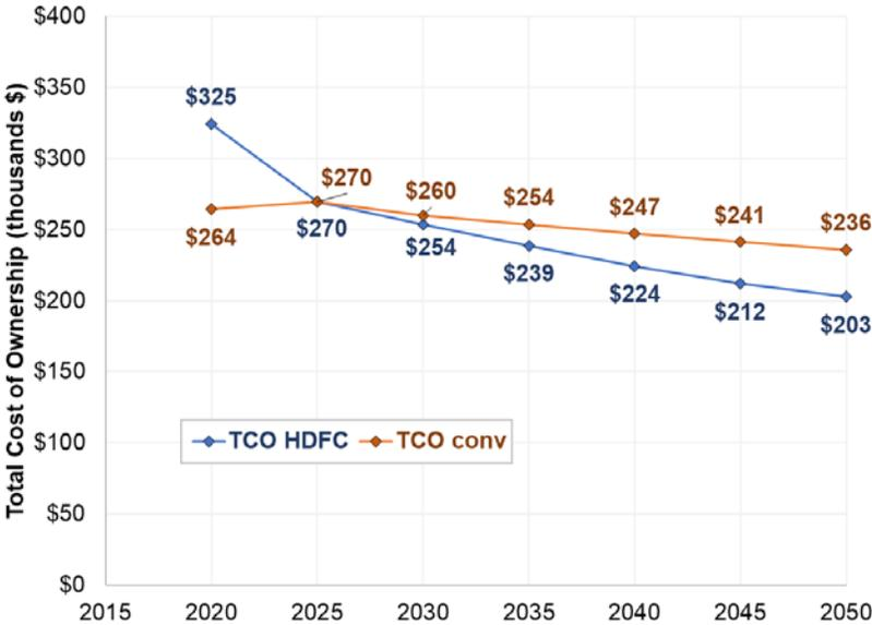
Figure 24. Total cost of ownership comparison for the conventional diesel and HDFC Class 8 yard tractor.
