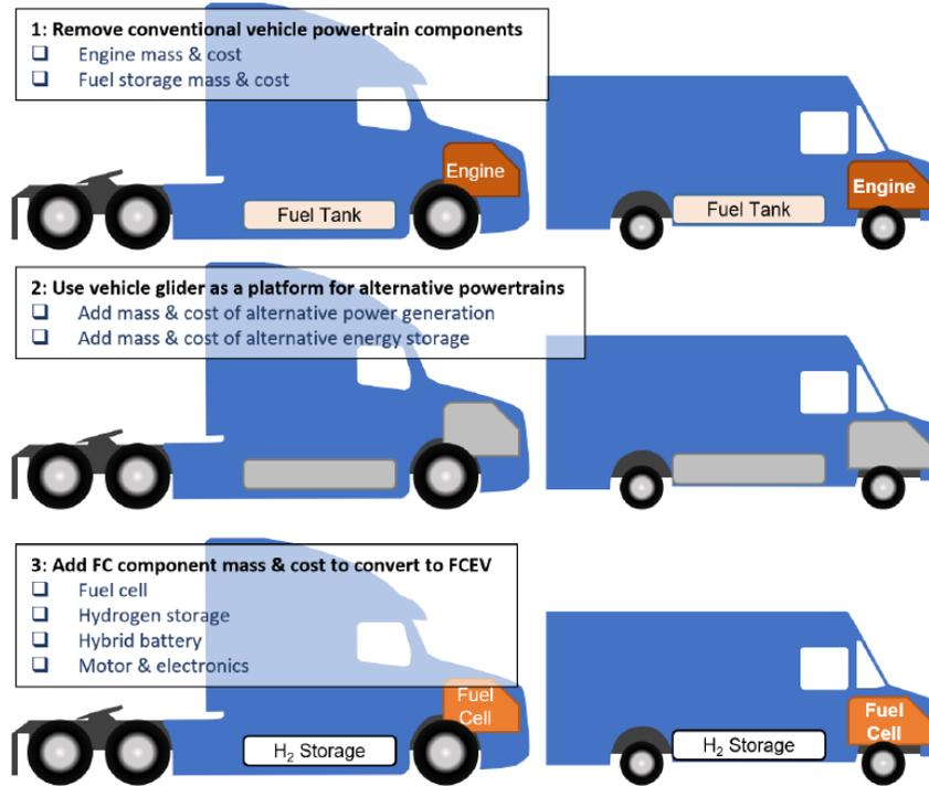
**Figure 8. Overview of the FASTSim methodology for estimating alternative powertrains for comparison to conventional diesel propulsion systems. Alternative powertrain components are sized to match the vocational requirements and performance of the diesel system (Hunter et al. 2021).**
