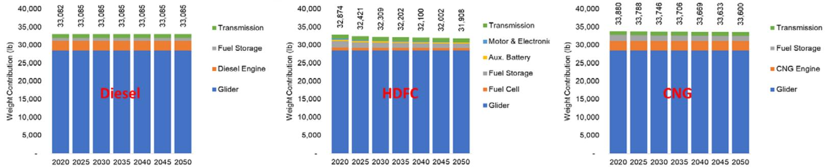
Figure 18. Weight breakdown for the Class 8 refuse truck for diesel, HDFC, and CNG powertrain options.
