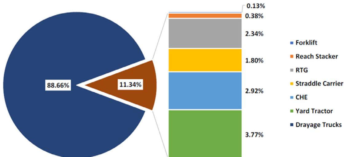
Figure 5. Energy consumption breakdown by port-side vehicle type at major U.S. ports (Steele and Myers 2019).
