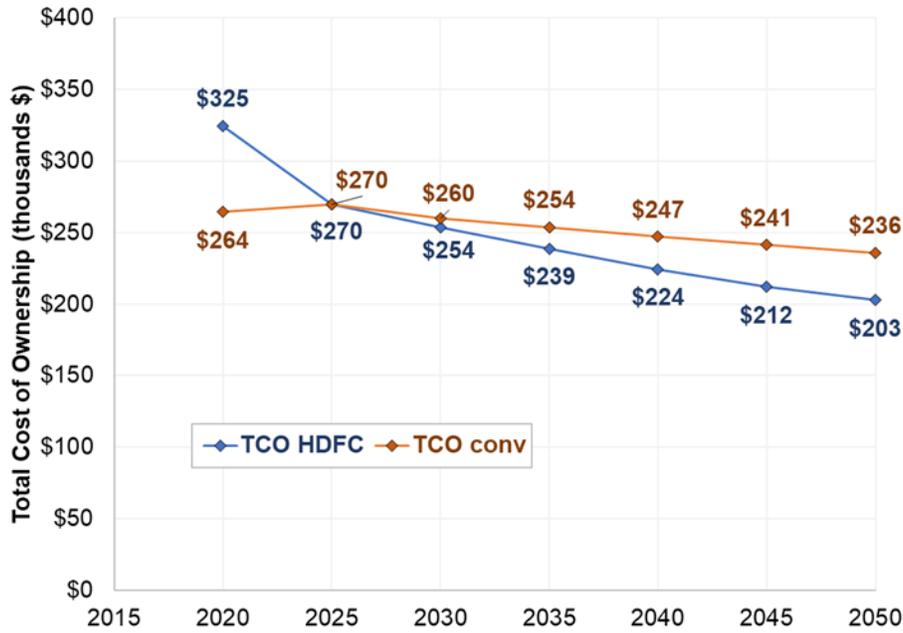
Figure 3. Total Cost of Ownership projections for technology years 2020 through 2050 for Class 8 Yard Tractors (200-mile range) for conventional diesel and heavy-duty fuel cell (HDFC) powertrains.
