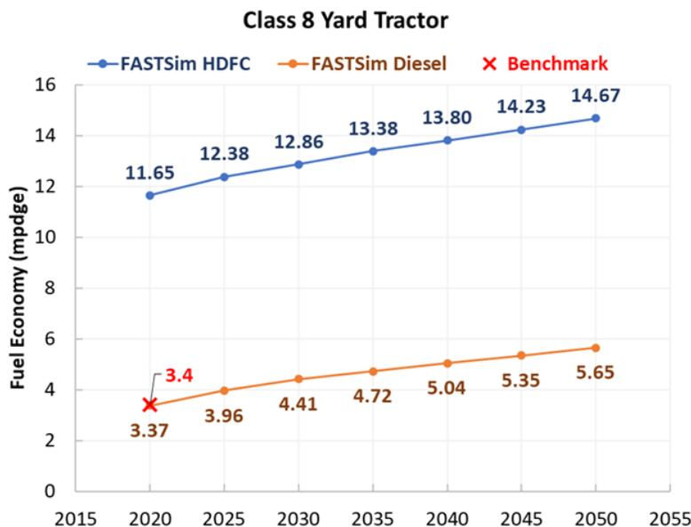
**Figure 1. Fuel economy projections for technology years 2020 through 2050 for Class 8 Yard Tractors (200-mile range) for conventional diesel and heavy-duty fuel cell (HDFC) powertrains.**
