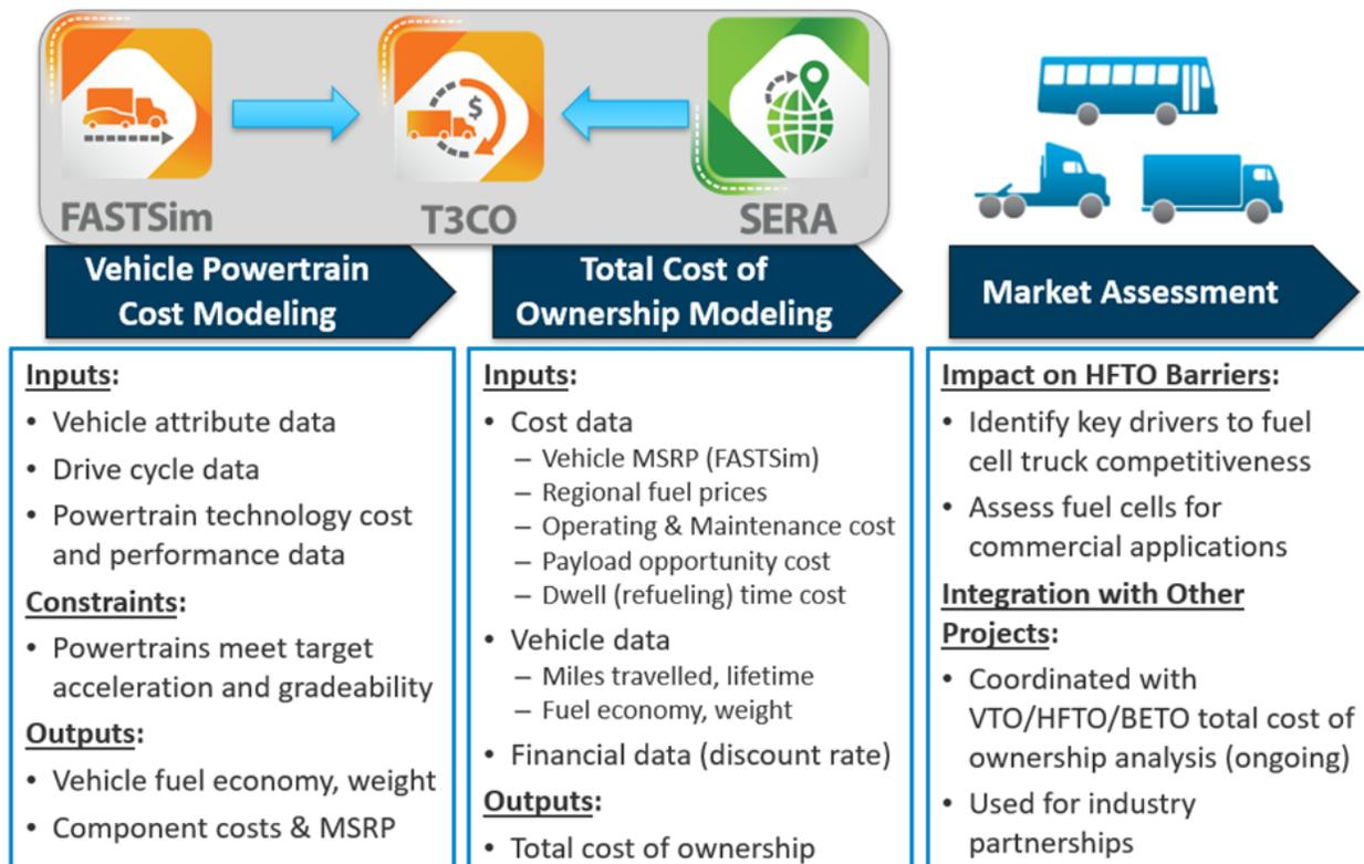
Figure 16. T3CO, FASTSim, and SERA modeling approach and flow process.
