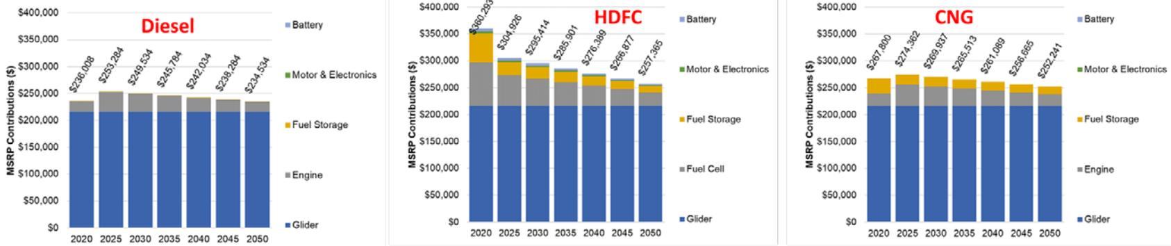
Figure 22. MSRP projections for conventional diesel, CNG, and HDFC Class 8 refuse trucks from 2020 to 2050.
