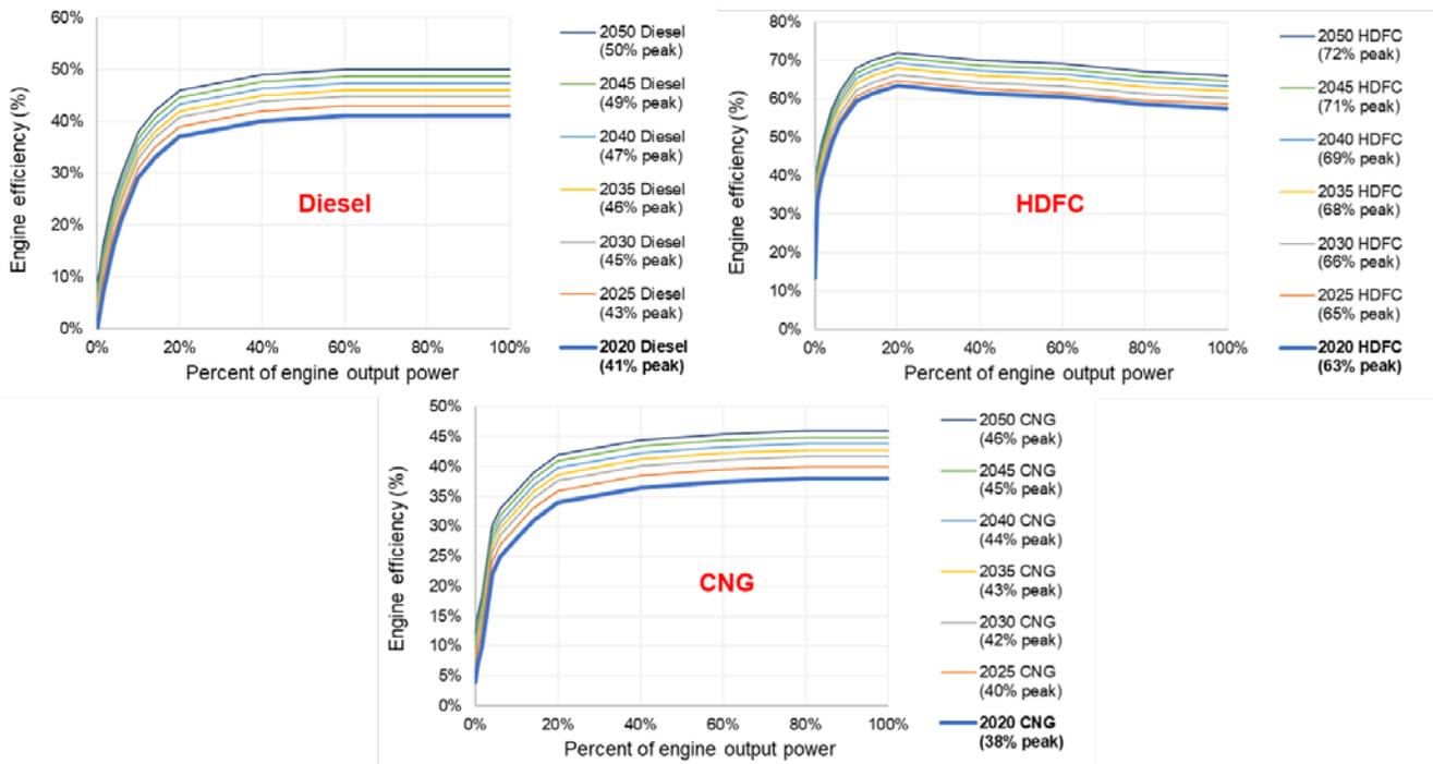
Figure 14. Class 8 yard tractor and refuse truck engine efficiency curve estimations for diesel, HDFC, and CNG (refuse truck only) powertrains based on representative duty cycle.
