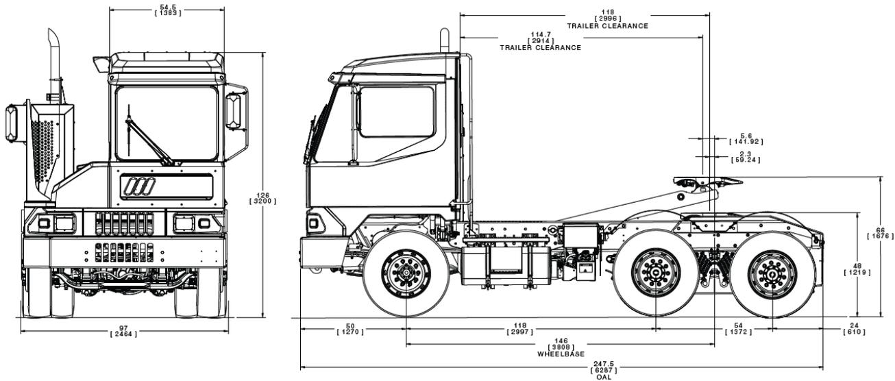
**Figure 9. Kalmar Ottawa 6x4 yard tractor size and dimensions used for FASTSim vehicle model.**
