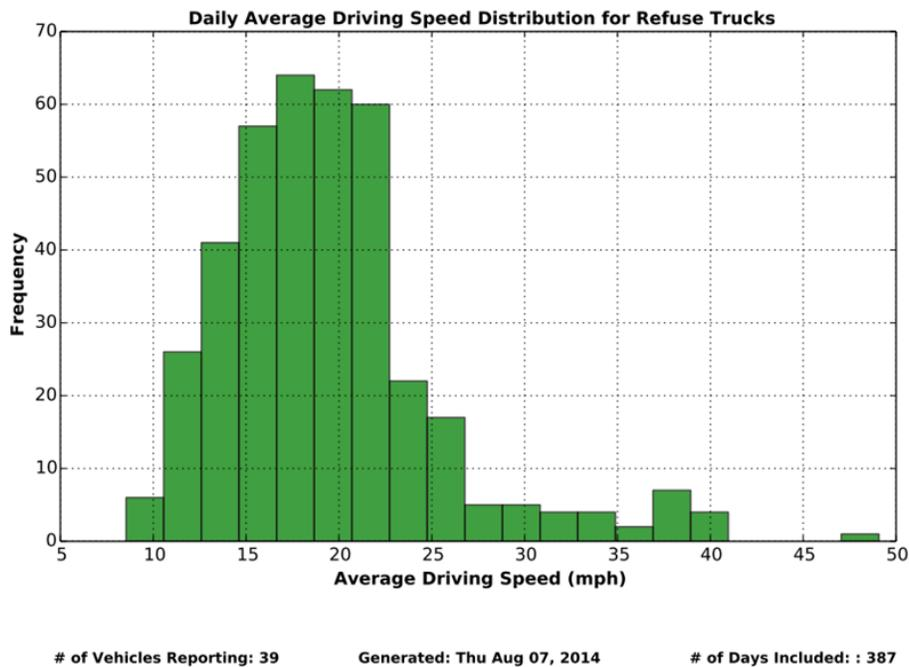
Figure 6. Distribution for daily average driving speeds for U.S. based refuse trucks. Data from NREL’s Fleet DNA database.
