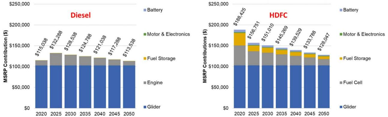
**Figure 21. MSRP projections for conventional diesel and HDFC Class 8 yard tractors from 2020 to 2050.**
