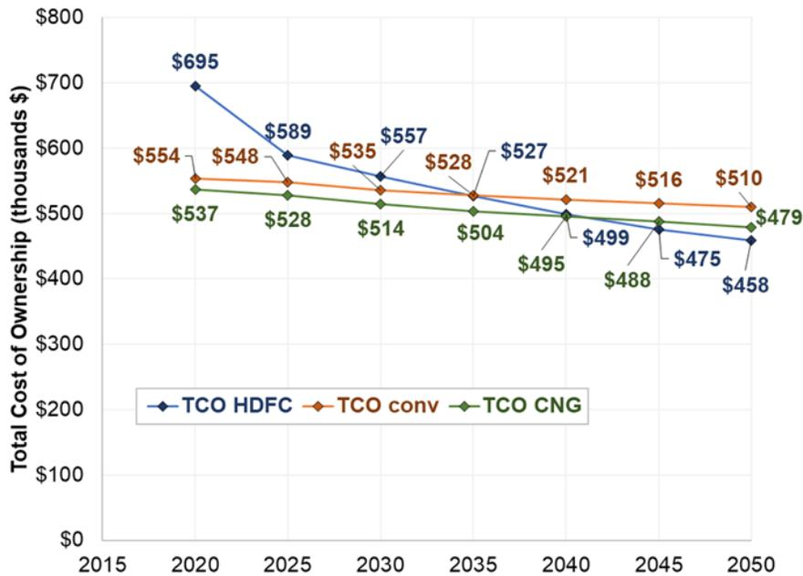
Figure 4. Total Cost of Ownership projections for technology years 2020 through 2050 for Class 8 Refuse Trucks (200-mile range) for conventional diesel, CNG, and heavy-duty fuel cell (HDFC) powertrains.
