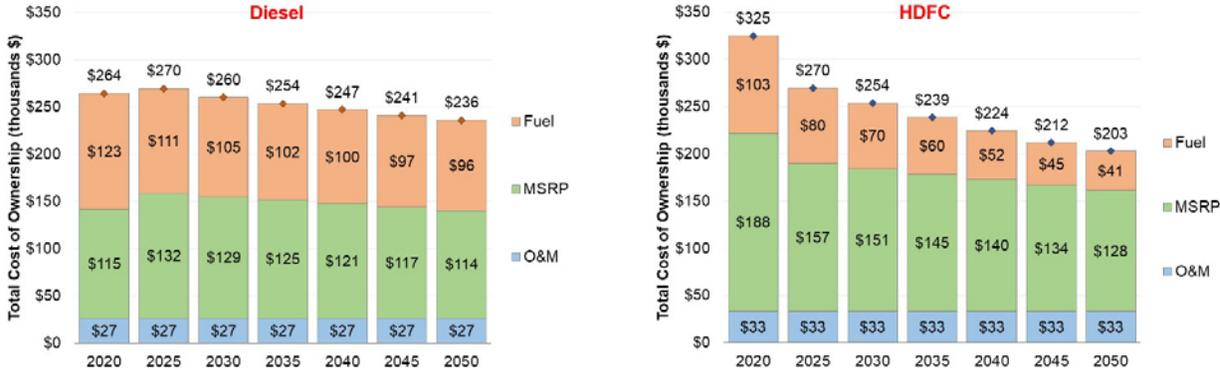
Figure 23. Total cost of ownership (TCO) projections for conventional diesel and HDFC Class 8 yard tractors projected from 2020 to 2050.
