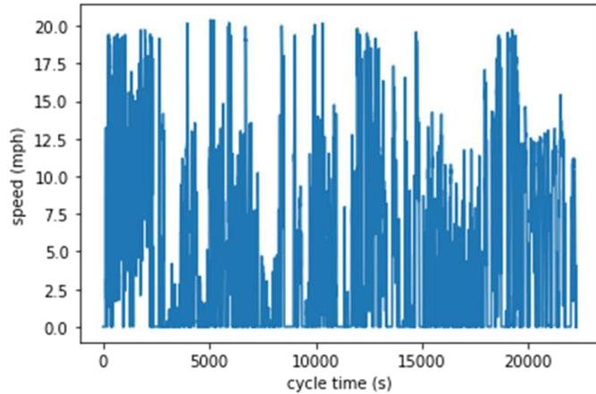
**Figure 12. Representative duty cycle for the Class 8 yard tractor with accompanying duty cycle attributes and metrics.**
