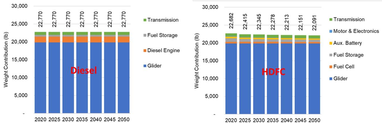
Figure 17. Weight breakdown for the Class 8 yard tractor for diesel and HDFC powertrain options.
