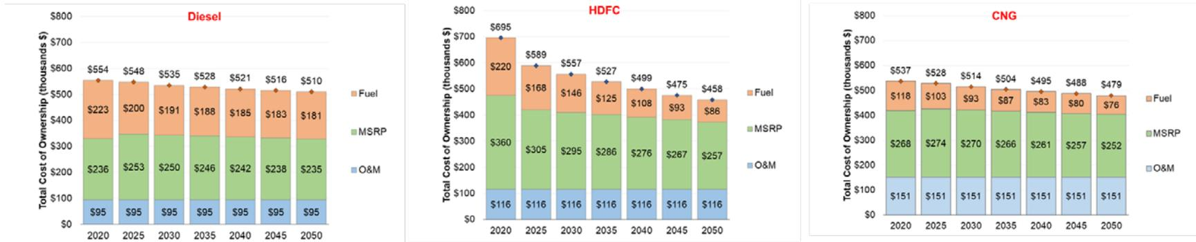
Figure 25. Total cost of ownership (TCO) projections for conventional diesel, CNG, and HDFC Class 8 refuse trucks projected out to 2050 (ultimate).
