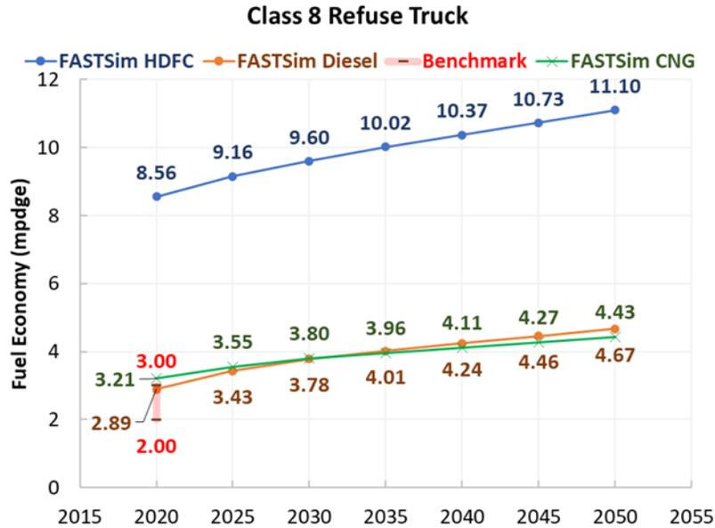
**Figure 2. Fuel economy projections for technology years 2020 through 2050 for Class 8 Refuse Trucks (200-mile range) for conventional diesel, CNG, and heavy-duty fuel cell (HDFC) powertrains.**
