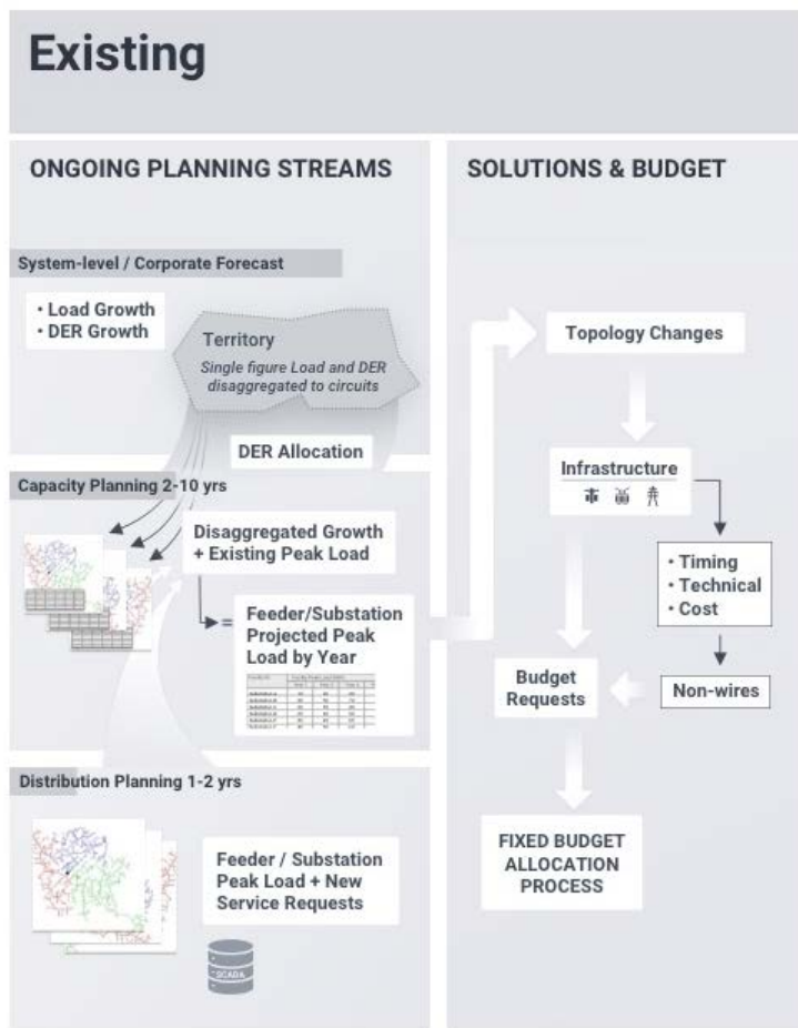
Figure ES-1. Existing distribution capacity planning framework where grid investments and deferral opportunities are determined by peak load forecasts in 2–10 years (left) and future distribution capacity planning framework with scenarios and probabilistic bottom-up load and DER adoption models, as well as multiple objectives and metrics driving the evaluation of distribution capacity solutions (right).
