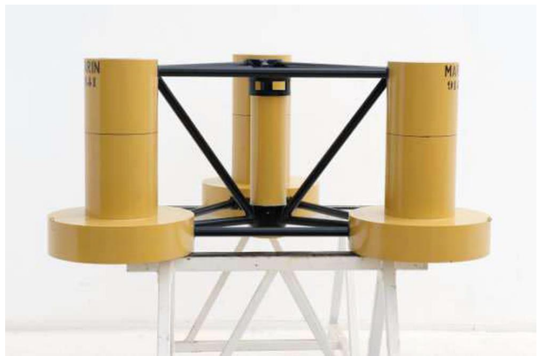
Figure 5. DeepCwind floating wind system design.
