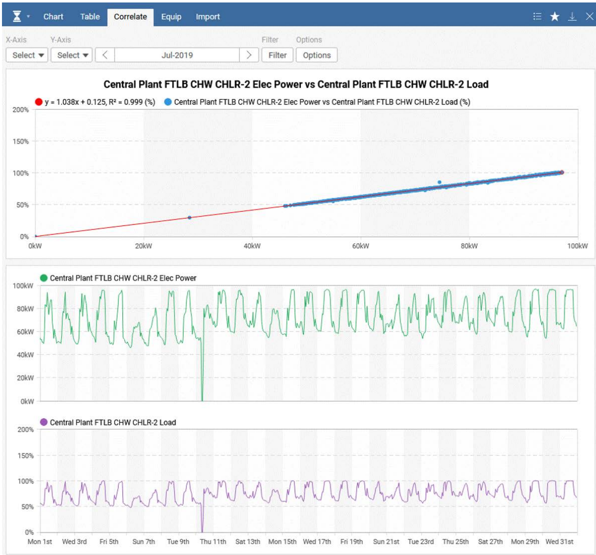
Figure 2. Correlation between FTLB Chiller 2 CHLR Elec Power and CHLR Load
