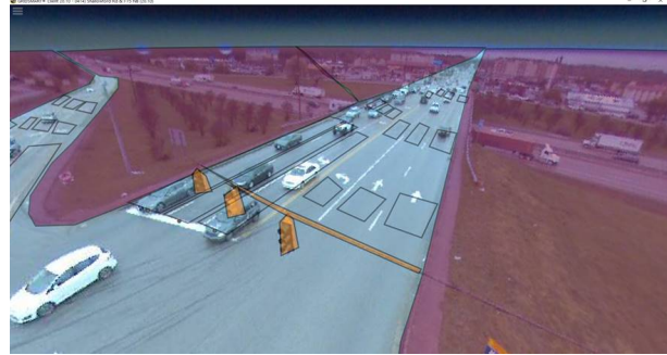
Fig. 6. Virtual detectors in a GridSmart camera view.
