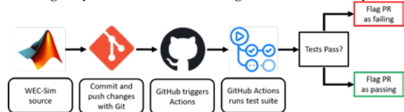
Fig.4 Testing workflow for WEC-Sim continuous interaction schema.
