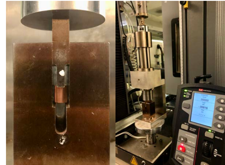
Shear fixture setup
