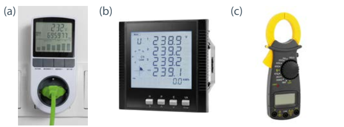
Figure 2. (a) Example plug-in digital power meter. Photo from iStock 175484325; (b) Example permanent circuit-level power meter. Photo from iStock 153688187; (c) Example temporary circuit-level meter. Photo iStock 111905131.
