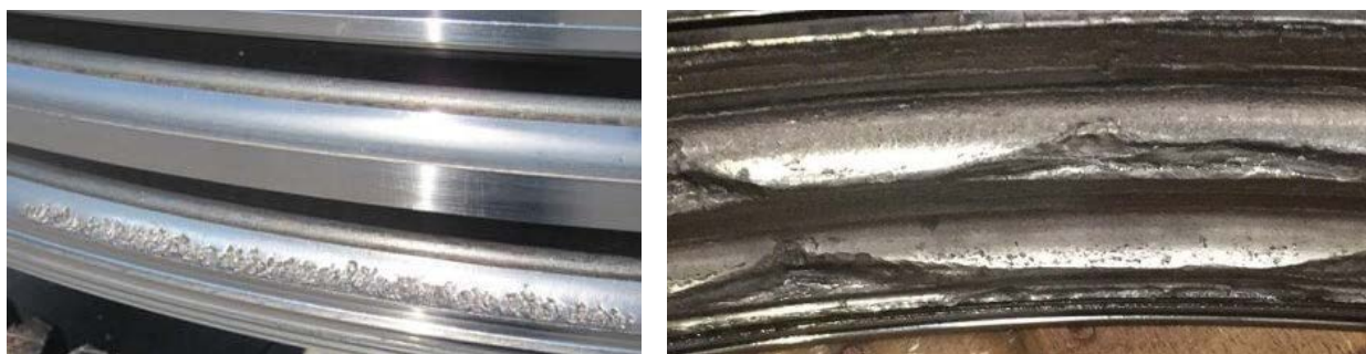
Figure 3. Example pitch bearing macropitting (left, [Dvorak 2016]) and contact truncation (right, [Bayles 2020]) damage
