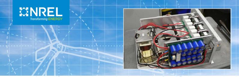
Windurance will produce an 80-kilowatt, three-phase version of this 25-kilowatt single-phase inverter developed by Intergrid. Image by Robert Wills, Intergrid
