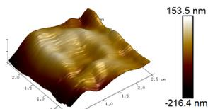
AFM topography image of a crater left in electrode after milling is completed.
