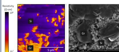
Domains in SSRM maps were identified using SEM-EDS, particle sizes, and known resistivity values<sup>2</sup>. Documented resistivity ranges are overlaid on resistivity histograms for each sample, below.
