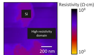
There are distinct higher resistivity domains in regions surrounding Si and Gr. The resistivity values measured in each of these domains were used to threshold the high resistivity volumes.
