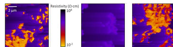
Multiple scans at random locations demonstrate that the GenF-cycled Si-graphite anodes had regions of surface graphite exposed, but Gen2 does not.
