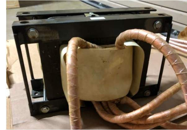
11"x 7" x 7", 175 kW, 20 kHz, Transformer, Based on Nano crystalline core and Litz (3/0) Winding
