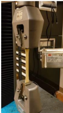
Fig. A.17: (Left) Mechanical testing of membrane specimens (middle). (Right) An example output of the results from the mechanical testing. Even though this schematic shows only monotonic, also creep and fatigue tests have been carried out. Conclusive results will be provided in the final report.
