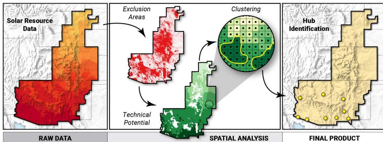
Figure 4. Workflow used by NREL to identify renewable energy zones
