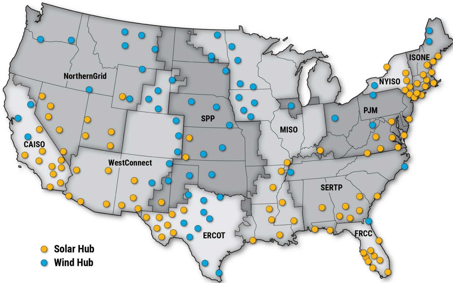
**Figure 5. Preliminary IREZ hubs by transmission planning region.**
