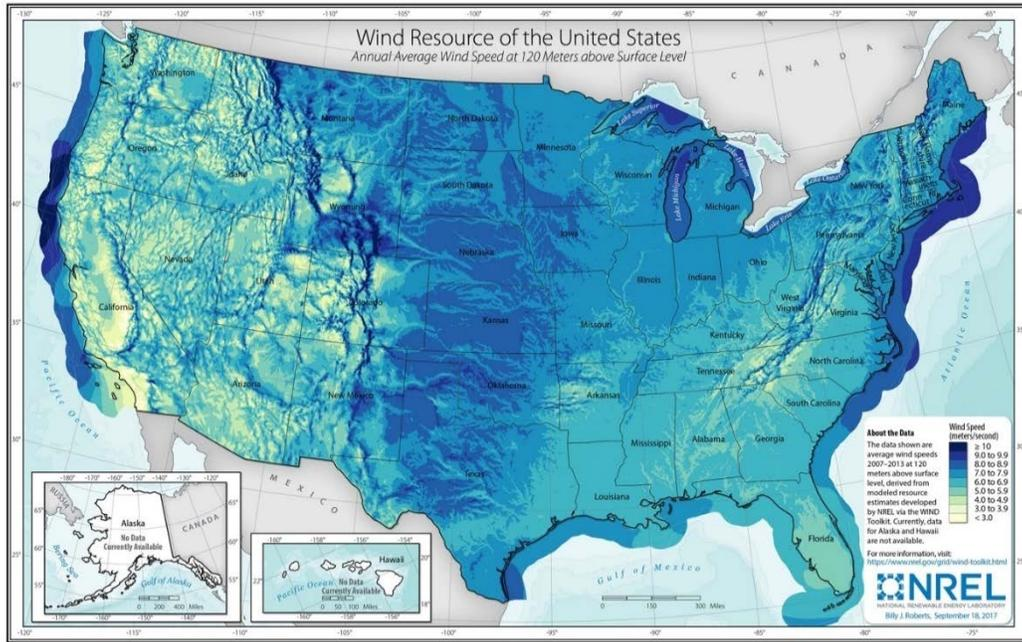
Figure 6. Wind resources at 120-meter hub height in the United States
