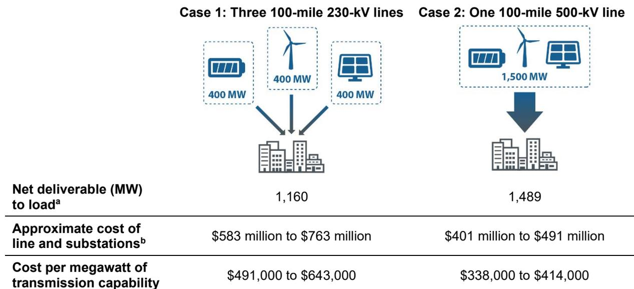
**Figure 2. Illustration of economies of scale for transmission**
