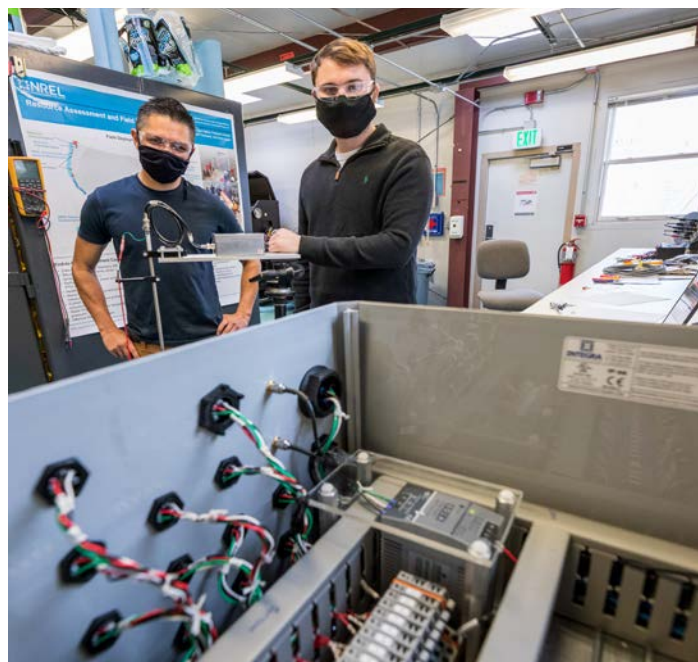
Water power researchers Andrew Simms (right) and Casey Nichols have been working on a customized data acquisition system for the University of Hawaii, which the team will use to collect data on their wave energy device's first offshore trial. Photo by Werner Slocum, NREL
