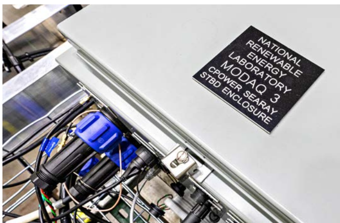
NREL's third Modular Ocean Data Acquisition system (MODAQ 3) was designed to serve the SeaRAY autonomous offshore power system, which makes and stores clean, carbon-free energy, and also shares data with the offshore vehicles it powers. Photo by Werner Slocum, NREL
