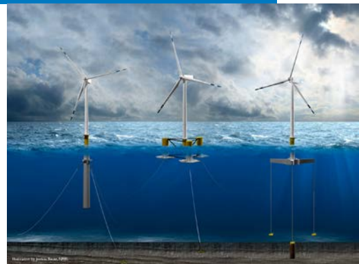
Example substructure types: (left to right) spar, semisubmersible, tension-leg platform (TLP).
