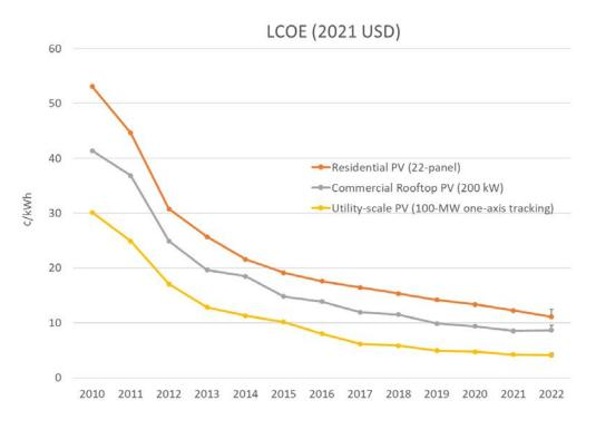
Figure 29. NREL-modeled PV LCOE over time
