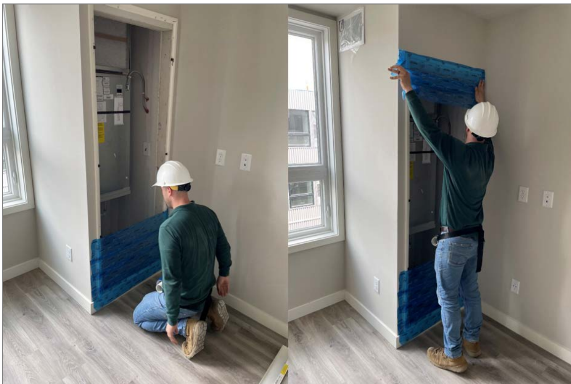
Figure 10. Supplemental test in modular unit 4 to determine air leakage through HVAC cabinet
