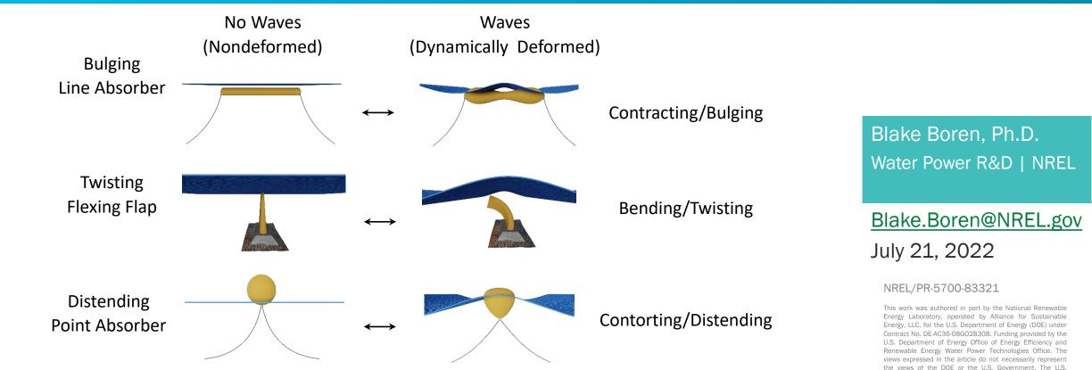
Three flexWEC archetypes - illustrating their methods of operation: ocean waves induce active deformations into the wave energy converter structures. The structures are made from distributed embedded energy converters (DEECs) that can convert those dynamic deformations directly into electricity; ocean wave energy conversion occurs throughout the structure without need to concentrate loads into a singular prime-mover or lone generator.
