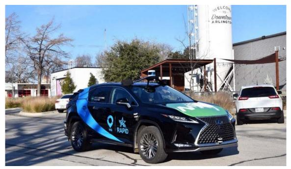
Figure 3-5. May Mobility deployed Lexus RX450h vehicles augmented by their ADS technology. Source: City of Arlington, Texas
