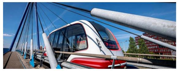
Figure 3-23. Third-generation AV ParkShuttle vehicle operating on the single-lane section of the bridge spanning across the expressway.
