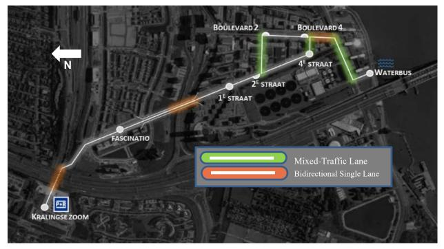
Figure 3-25. Rivium Business Park AV shuttle alignment for the complete Phase 3 expansion, with mixed-traffic segments and single-lane segments shown.
