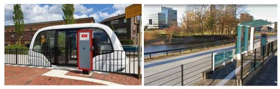
Figure 3-27. Precision docking allows wheelchair-level platform boarding at station berths. Source: 2getthere, a company of ZF
