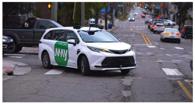
Figure 3-9. The Toyota Sienna MaaS vehicle will be equipped with the May Mobility ADS, using Via's fleet dispatching system to provide point-to-point, dynamically pooled rides.
