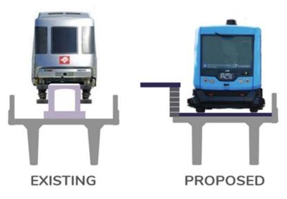
Figure 3-13. Concept for removing the monorail beam to return the structure to rubber-tired automated vehicle technology similar to the original vehicle form factor.
