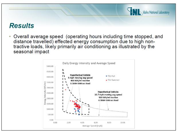
Figure 3-20. Final results of the Idaho National Laboratory energy use data collection for the TSU shuttle operation.
