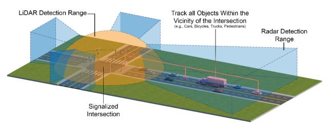
Figure 6-2. Next-generation traffic control has multiple sensors at IRI intersections.
