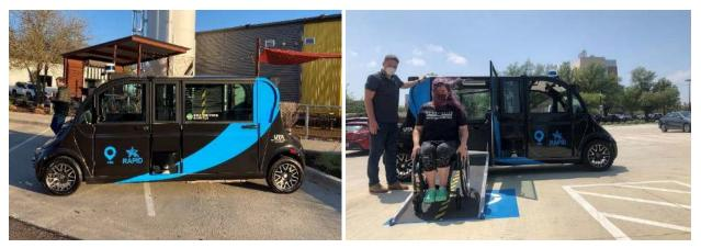
Figure 3-6. May Mobility's Polaris GEM AV shuttle for wheelchair-accessible service.
