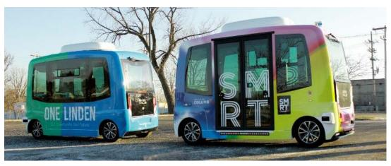
Figure 3-2. EasyMile Gen 3 vehicles that operated the Linden LEAP service.
