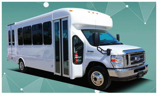
Figure 2-3. Houston University District Phase 2 battery-electric paratransit bus—Phoenix Motorcars Z400 electric shuttle.
