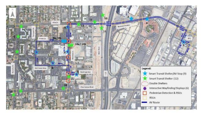
Figure 3-11. GoMed AV circulator travel route, Smart Transit Shelter, pedestrian detection, and connected vehicle roadside unit locations.
