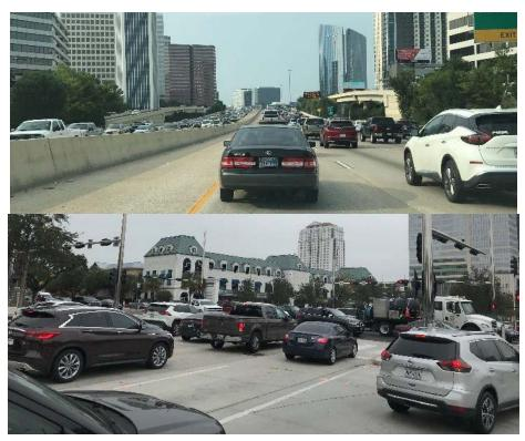
Figure 4-3. Traffic congestion on the capacity-limited freeway bisecting the urban district actually forces congestion back through the arterial streets that intersect the freeway.
