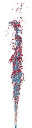
Lagrangian fuel sprays in PeleLM eX (droplets colored by T) Ariente et al., in prep, 2022
