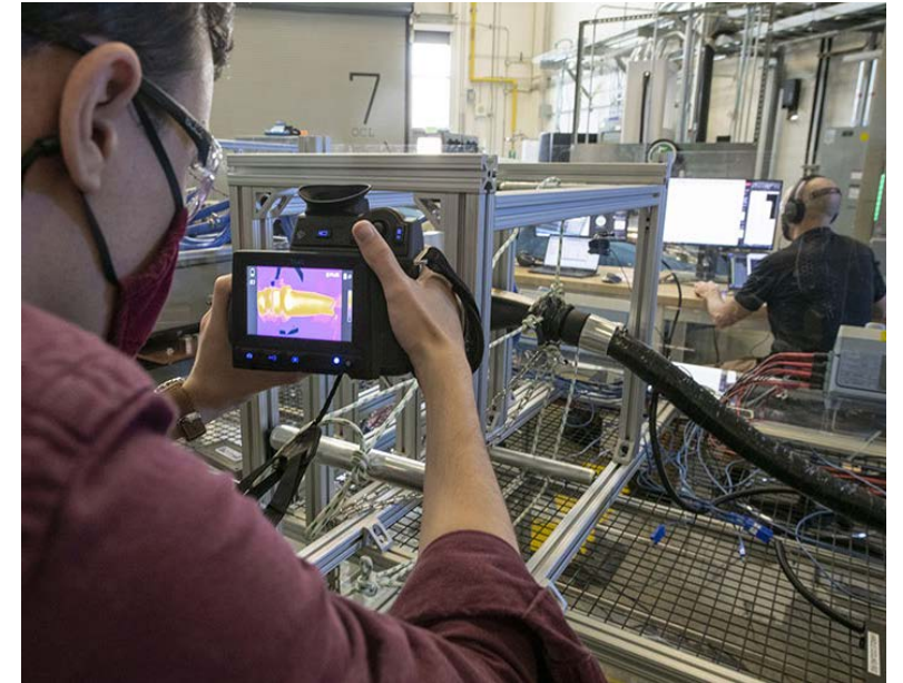
Researcher captures thermal image of an MCS charging system during evaluation at the MCS 2 nd Event in Fall of 2021. (Photo by Dennis Schroeder, NREL)
