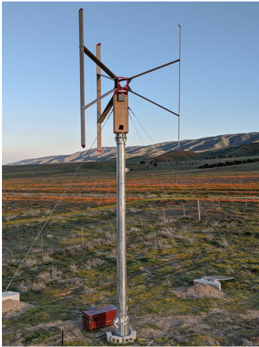
Figure 9. XFlow's 5 kW prototype VAWT at the Field Laboratory for Optimized Wind Energy in Lancaster, California.
