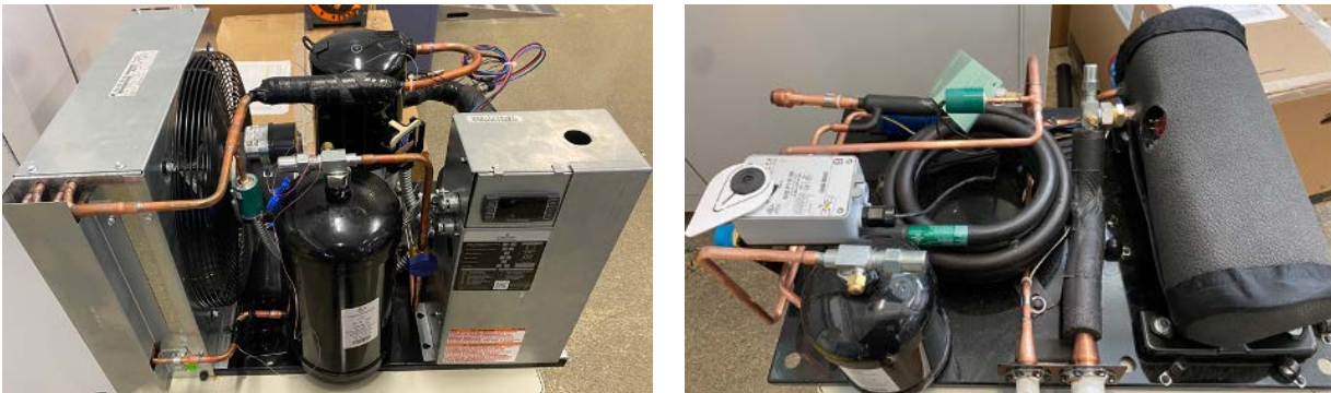
Figure 2. Baseline air-cooled condenser (left) and high-efficiency liquid-cooled energy conserving condenser (right). Photos by Alexander Bulk.
