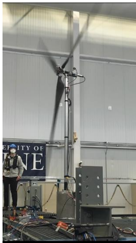
Figure 1. 1:70 scale model of IEA Wind 15-MW turbine.
