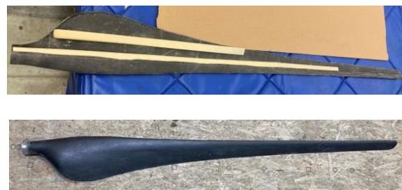
Figure 6. Model blade as built, Stiffening foam spar placement shown in top figure
