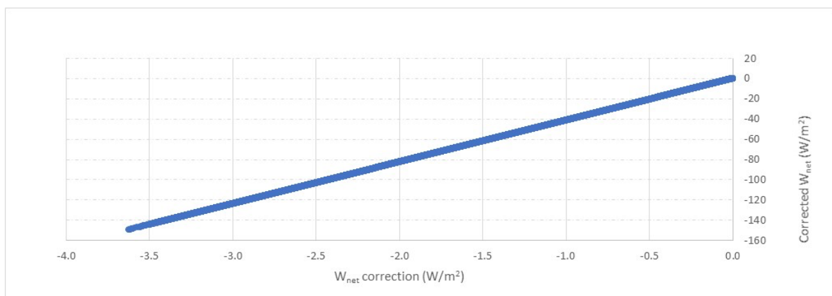
Fig. 11. Corrected W_{\text{net}} versus the W_{\text{net}} correction PIR at the SGP station sgpbrcC1
