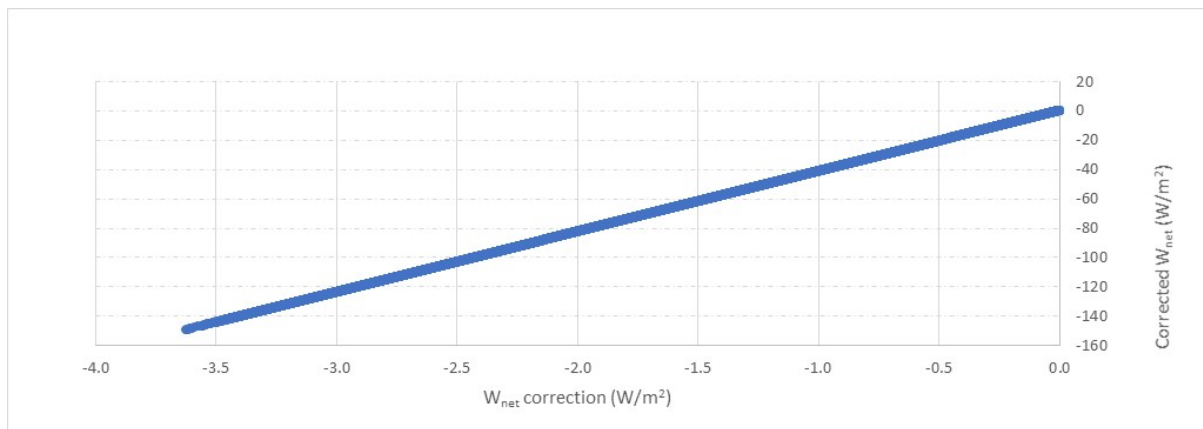
Fig. 9. Corrected W_{\text{net}} versus the W_{\text{net}} correction PIR at the SGP station sgpsirsE13
