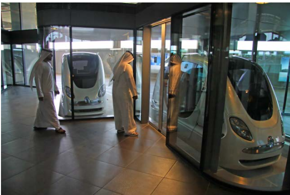
Masdar City PRT station configuration Source: 2getthere, a subsidiary of ZF Group
