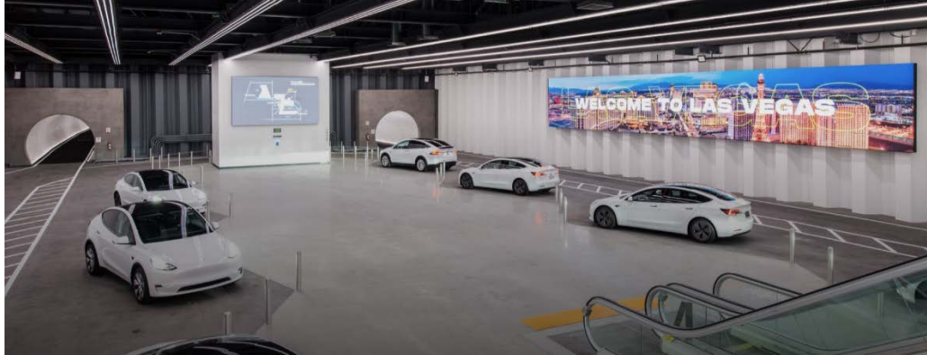
Figure 7. Bidirectional station with parallel berths at LVCC Loop System Central Station.
