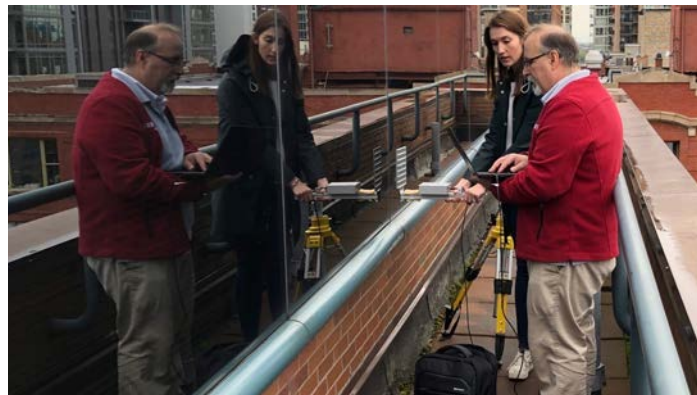
The Sonic Leak Quantifier (SonicLQ) uses sound waves to locate and size air leaks in building walls, doors, and windows. Photo Dr. Ralph T. Muehleisen, ANL.
