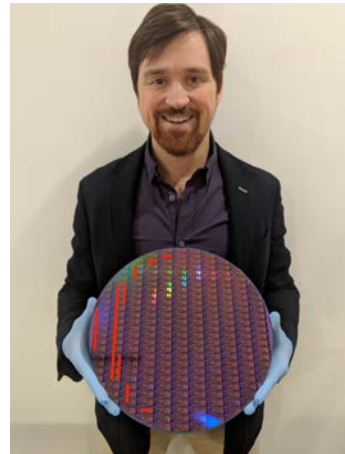
Iris Light founder Chad Husko holding a 12-inch (300-mm) silicon wafer composed of hundreds of chips. Iris Light on-chip lasers are made by depositing proprietary photonic ink onto the surface of a pre-patterned wafer like the one shown here. Photo by: Mary Reid Ervin.
