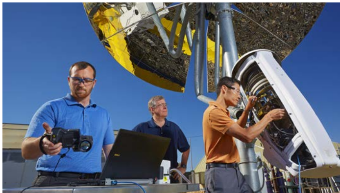
PNNL researchers Paul Armatis, Bob Wegeng, and Richard Zheng shown with the Solar Thermochemical Advanced Reactor System, which uses concentrated solar power to convert natural gas into more valuable fuels, including hydrogen for fuel cell cars. Photo by PNNL.
