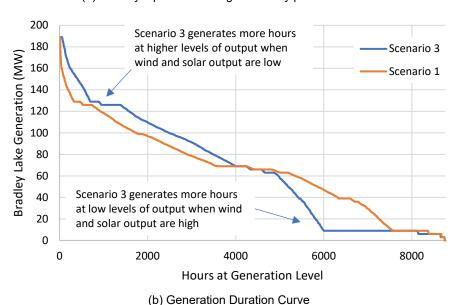
Figure 9. Operation of the Bradley Lake hydroelectric plant
