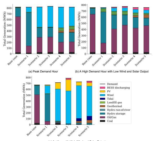
(c) An Hour with High Wind and Solar Output
