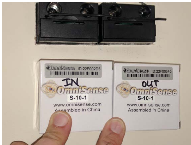
Figure 13. Typical moisture sensor placement in SPS wall showing interior surface and exterior surface panel depths
