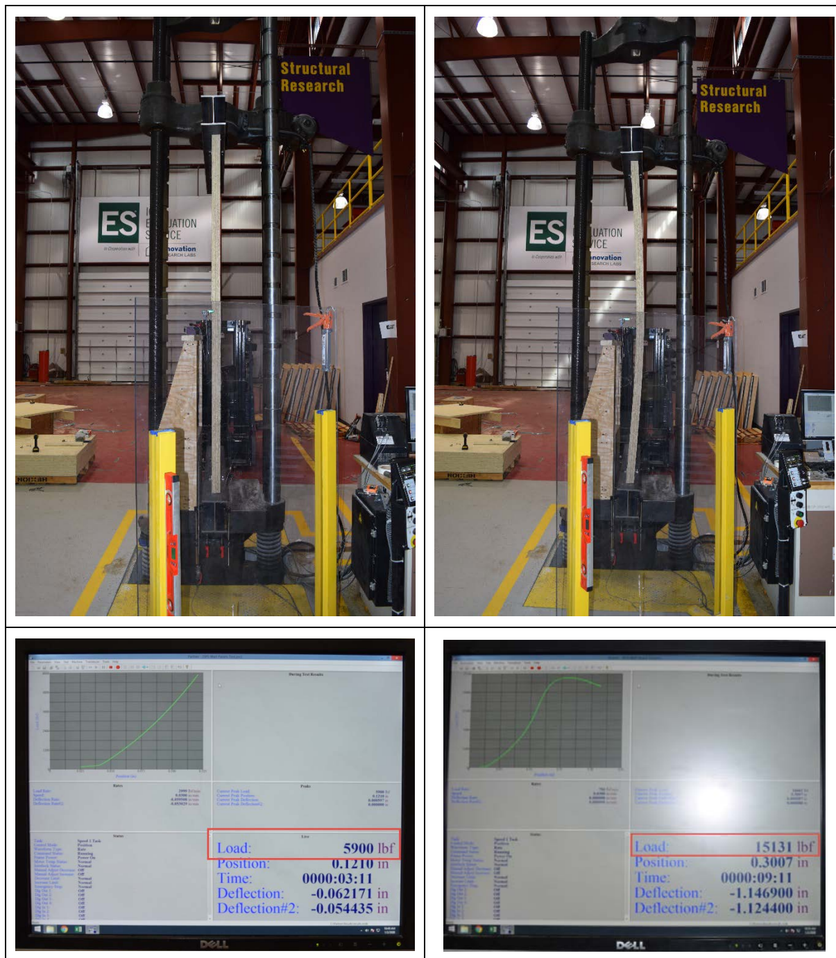
Figure F-3. At 15,000 lbs of force, bowing was observed at the midline of the 2-ply SPS specimens
