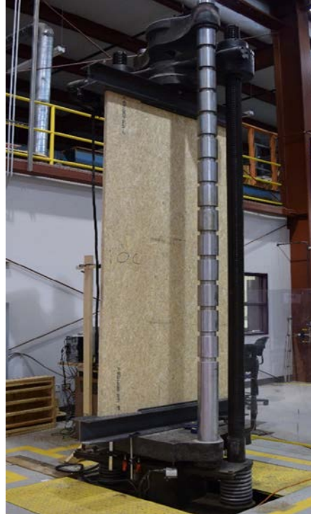
Figure 16. Universal Test Machine test setup per ASTM E72
