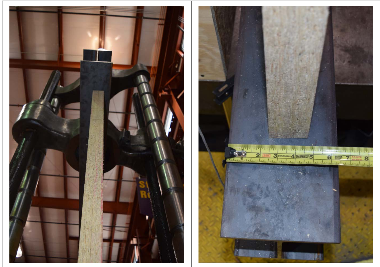
Figure F-2. Flanges bolted to the I-beams allow the specimen to be loaded into the UTM at the 1/3 distance prescribed by E72 to force the direction of buckling
