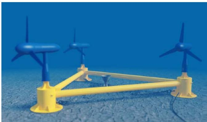
This illustration shows how the Verdant Power TriFrame is installed at the bottom of New York City's East River. NREL has been working with Verdant Power since 2008 to develop new tools for marine energy applications
