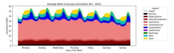
Figure B-17. Average weekly dispatch for each generation technology in January: Reference Scenario
