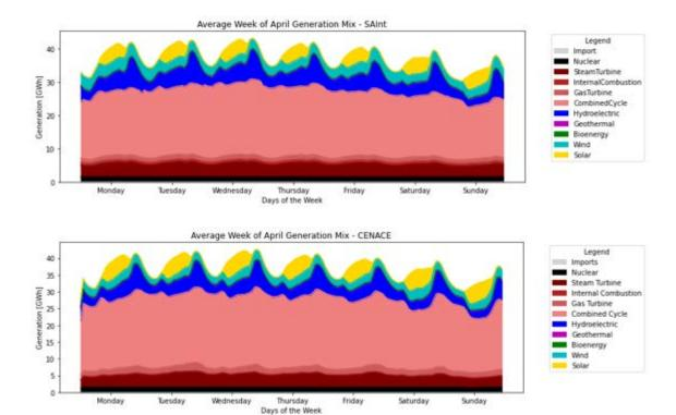
Figure A-2. Average Weekly Dispatch Per Generation Technology for April
