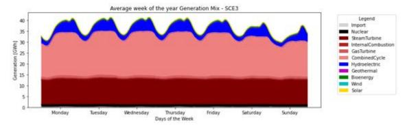
Figure B-16. Average weekly dispatch for each generation technology: Scenario 3
