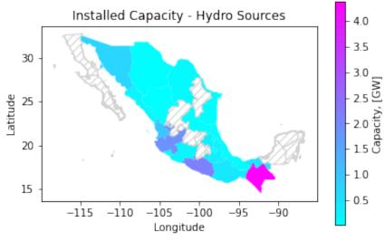
Figure 4. Installed operational hydroelectric generation capacity per Mexican state.
