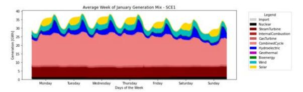
Figure B-18. Average weekly dispatch for each generation technology in January: Scenario 1
