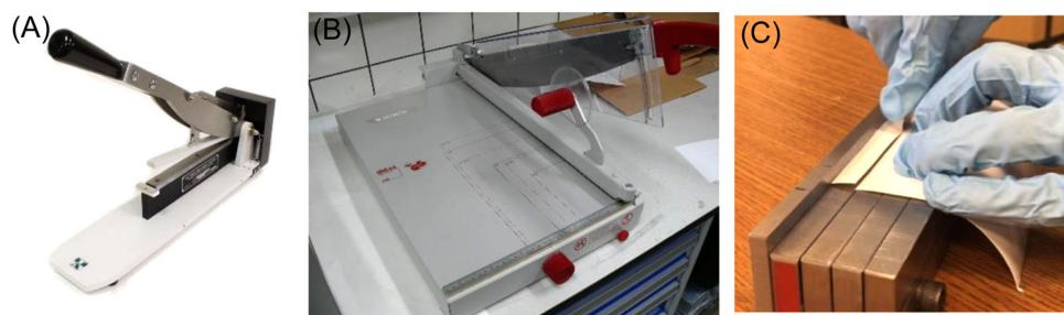
FIGURE 1 Cutting method photos. (A) Tensile specimen punch (JDC precision sample cutter) (B) paper cutter, and (C) fresh razor blade
