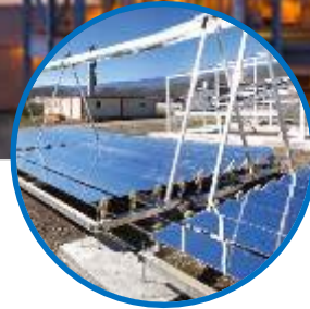
Linear Fresnel collectors (LFCs) coupled with phase change material (PCM) thermal energy storage (TES) for Food & Beverage Industry
