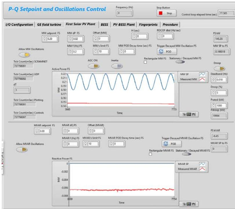
**Figure 61. Main control screen for the P-Q set points and oscillation control**
