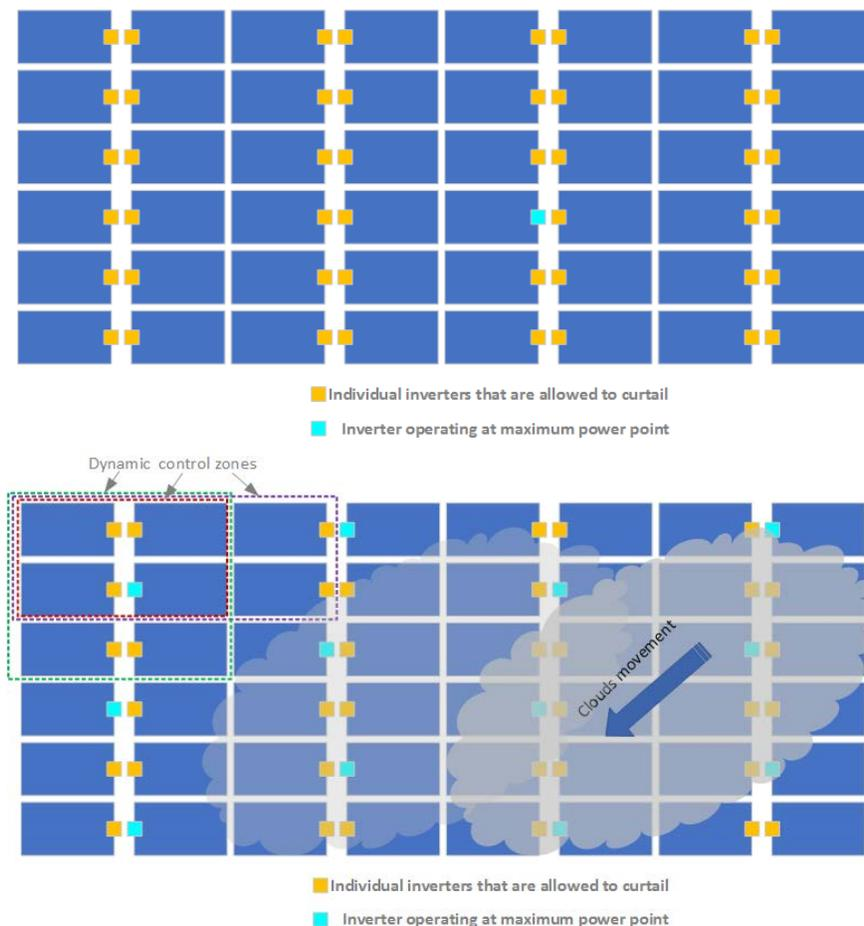
**Figure 102. Large PV power plant divided into control zones during cloud conditions**
