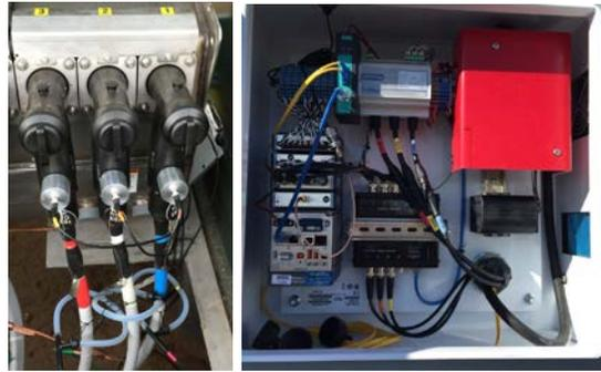
**Figure 75. Hardware in each medium-voltage DAS sensing node: (left) voltage and current sensors; (right) data conditioning built around the National Instruments' cRIO-9030 platform. Photos by NREL**
