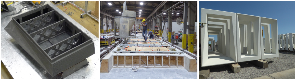
Figure 14. Additive manufacturing has been demonstrated successfully for precast concrete forms of building facades. Avenues to employ advanced manufacturing techniques, such as additive manufacturing, for energy-efficient window-to-facade integration merit additional investigation.
