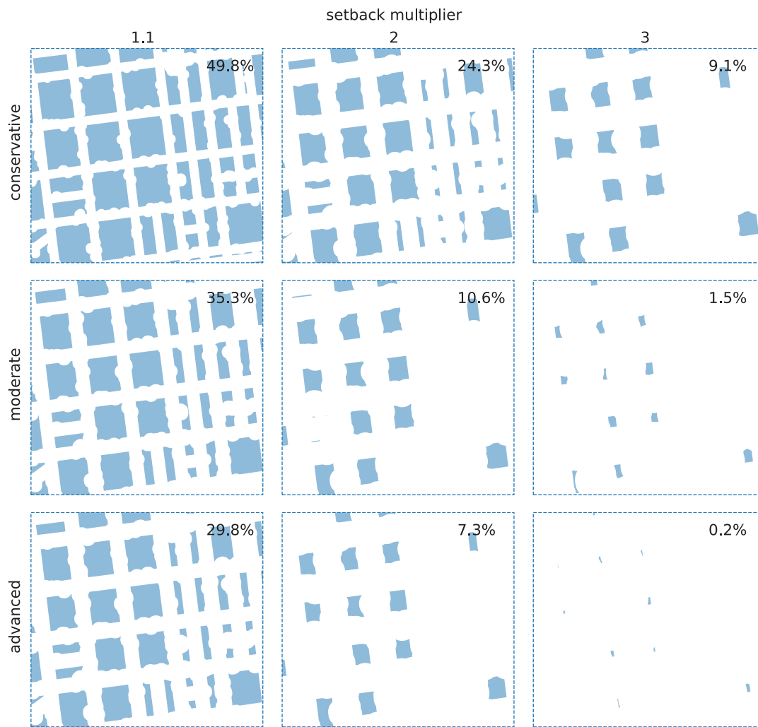
Fig. 4. The available area remaining in the wind plant domain with different setback requirements from various features. Each column represents different setback requirements of 1.1, 2, and 3 times the turbine tip height, and each row represents a different turbine design (corresponding to the turbines represented in Fig. 3). The shaded blue areas represent the areas where turbines can be built, and the percentage in the top right corner of each subfigure shows the percent of the total land area still available after applying the setbacks.
