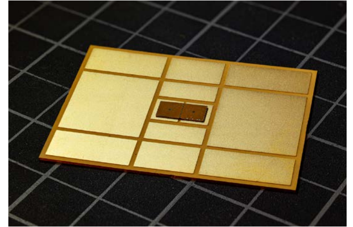
IIC Package on Dupont ODBC Substrate
