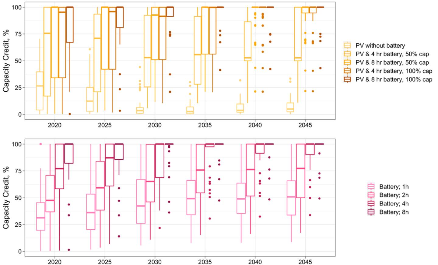
**Figure 7. Capacity credit of PV + battery and stand-alone battery configurations across the entire Western Interconnection for the High RE, Low Cost scenario**
