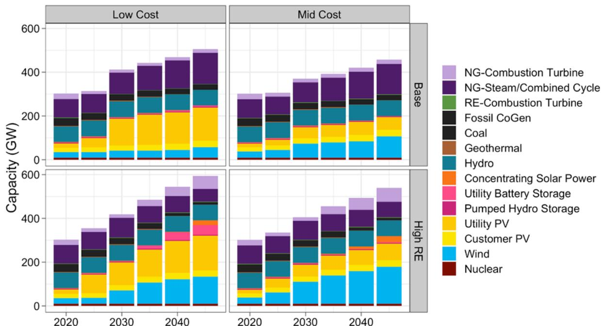
**Figure 11. Installed capacity across WECC in scenarios without PV + battery**
