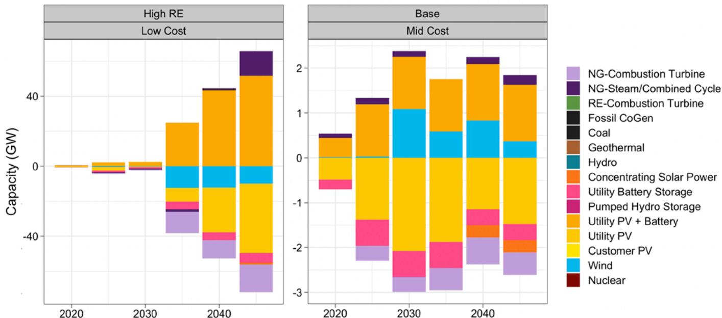
**Figure 12. Changes in installed capacity with the addition of PV + battery as a technology option**
