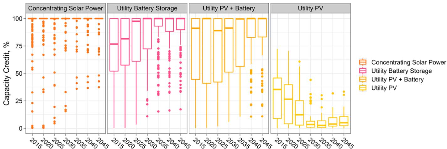
**Figure 6. Capacity credit of all technology configurations of utility-scale solar and storage options (not necessarily all installed) in the High RE, Low Cost scenario, aggregated across all configurations and all regions in the Western Interconnection**
