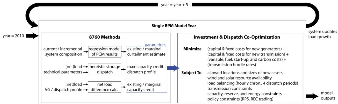
**Figure 3. Algorithmic structure of RPM**
