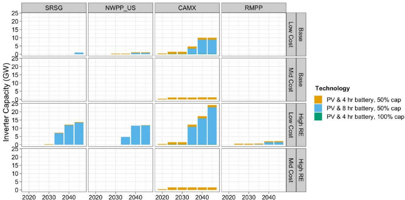
**Figure 13. PV + battery configurations installed by scenario and NERC region**
