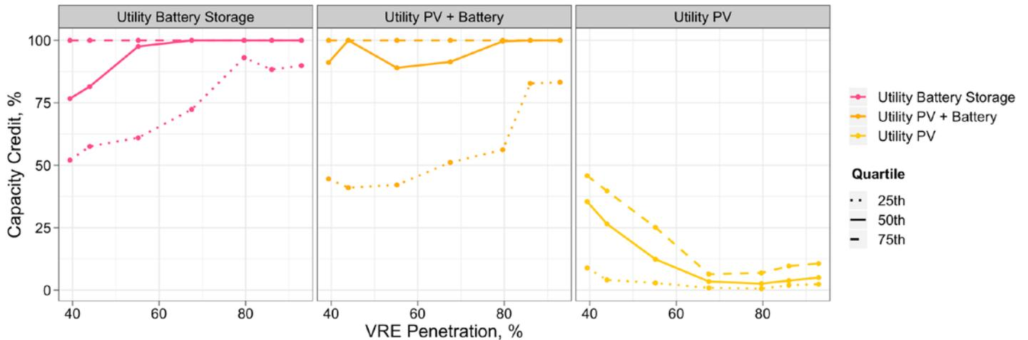
**Figure 8. Capacity credit for all U.S. NERC regions in the High RE, Low Cost scenario, relative to the variable renewable deployment**
