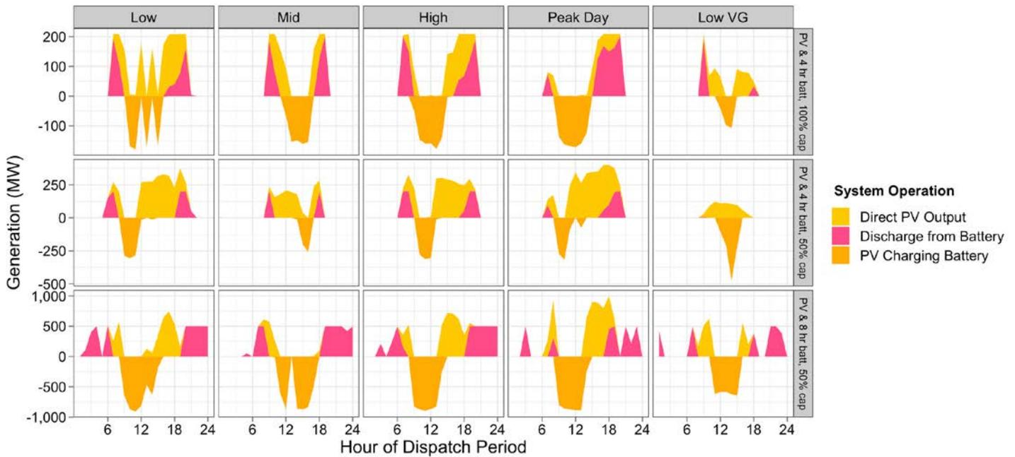
**Figure 10. Hourly PV + battery dispatch by configuration from the High RE, Low Cost scenario 2045**
