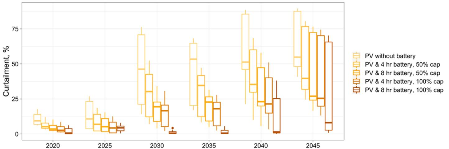
**Figure 9. Curtailment of PV + battery technology configurations across the Western Interconnection for the High RE, Low Cost scenario**
