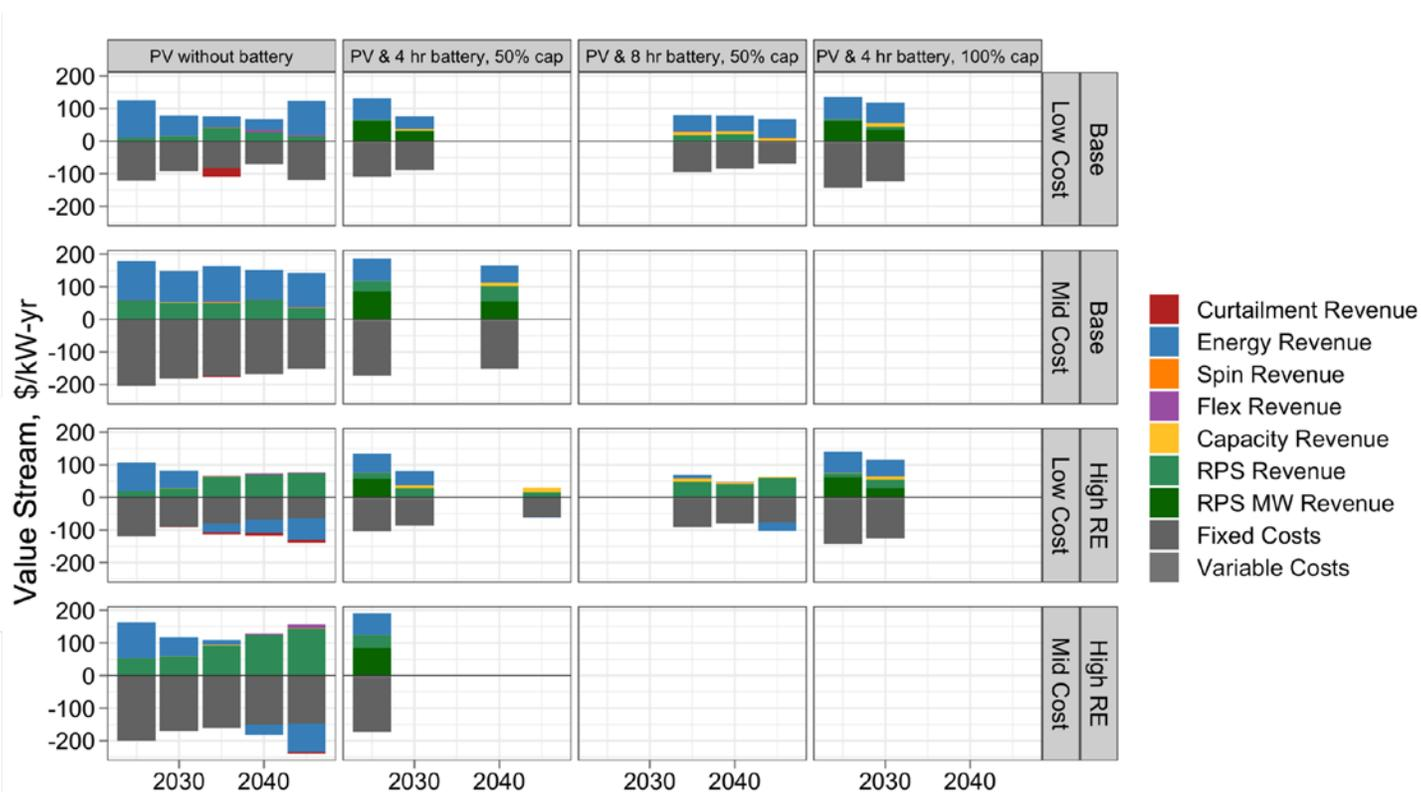
**Figure 14. Value streams for PV + battery technologies compared to stand-alone PV for all scenarios, aggregated for all regions**
