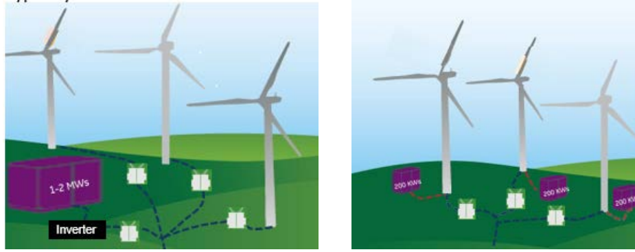
a) Central storage at the plant level b) Integrated storage at each turbine
