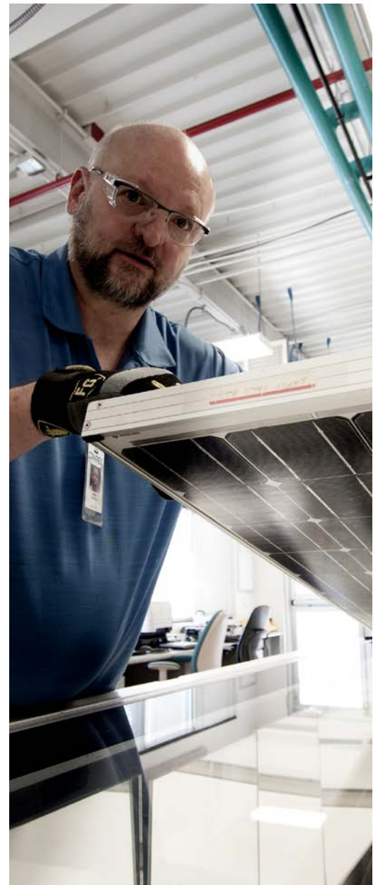
Indoor testing of PV modules at NREL. Photo by Nikos Kopidakis
