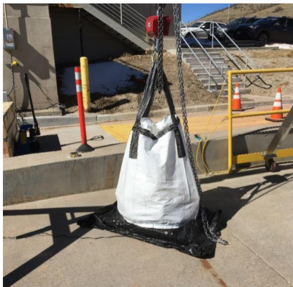
Fig. 1. Participant's product undergoing the load test. The PV module and load are contained in cloth bags for safety purposes in the event of a PV module or load testing method failure.
