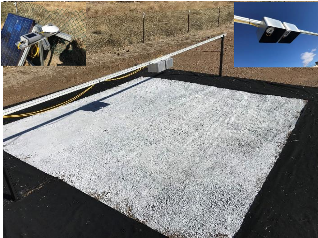
Fig. 2. Albedometers located over the center of the test plot. Expanded view of the GRI instruments shown in upper right. GHI instruments shown in upper left.
