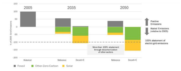
By replacing significant direct fossil fuel use in the buildings, transportation, and industrial sectors, the Decarb+E scenario abates more than 150% of the electric grid's 2005 carbon emissions.
