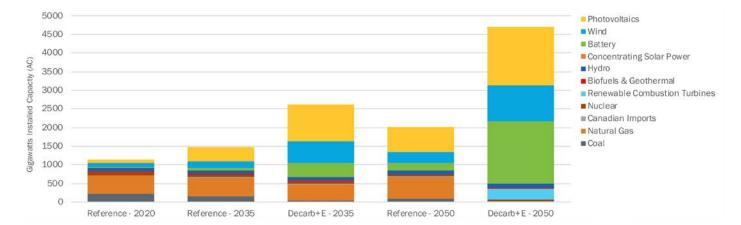
Generation capacity on the U.S. electric grid under the study's three scenarios over time. Solar, wind, energy storage, and renewably fueled combustion turbines (CTs) all play a key role in decarbonization.
