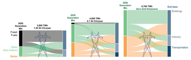
Grid mixes and energy flows in 2020, 2035, and 2050, as envisioned in the Solar Futures Study. Newly electrified loads from buildings, transportation, and industrial sectors mean that the electric grid will deliver more energy in 2035 and 2050. This energy will come almost entirely from solar and other zero-carbon sources.
