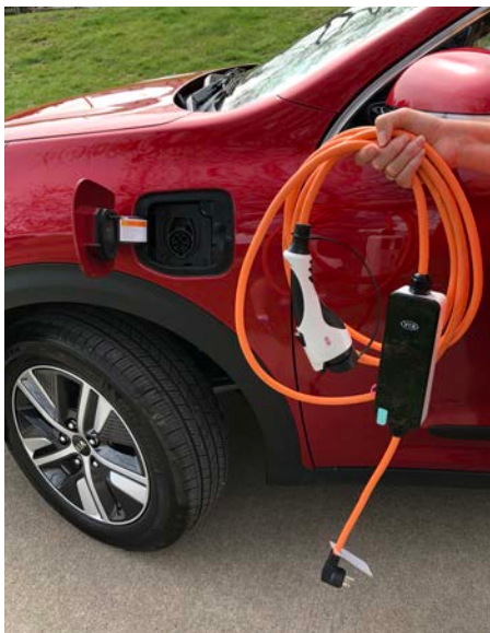
Getting started with an EV is easy thanks to the charging “cordset” that comes with most vehicles. Photo by Erik Nelsen, NREL 64277.
