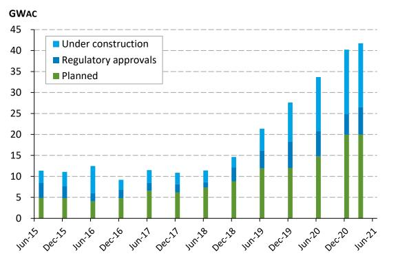
According to EIA data, the U.S. PV project pipeline of utility-scale PV projects continues to hit record highs, with 15  $GW_{AC}$  of projects under construction, 7  $GW_{AC}$  having received regulatory approval, and 20  $GW_{AC}$  planned as of March 2021.
